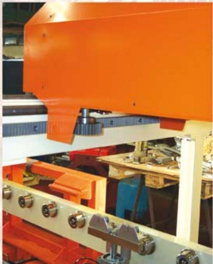
The Horizontal Automatic Tile Handling System has been designed for automatic transfer of steel trays containing green and dried tiles.
