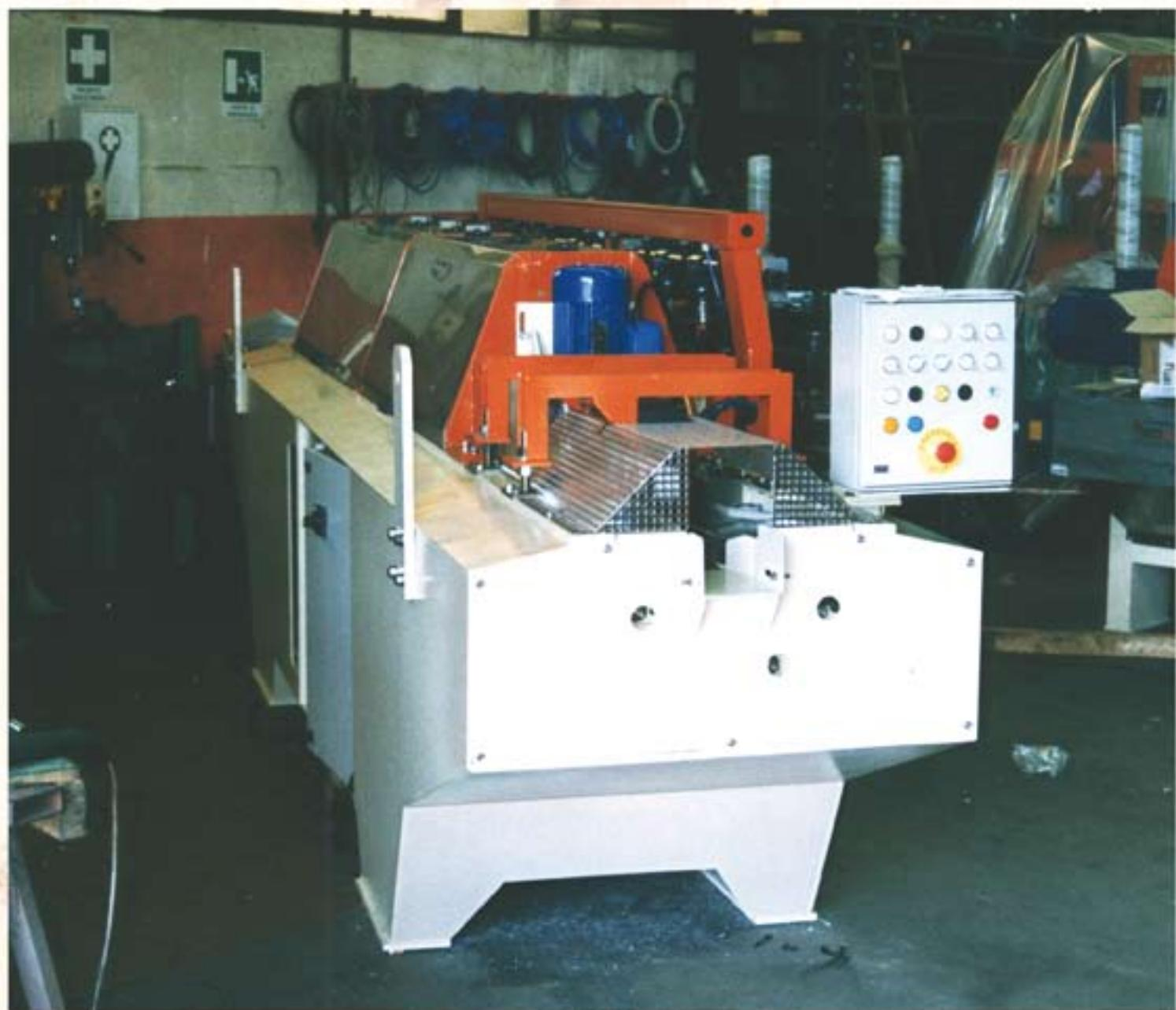
The Automatic Bevelling Splitting Machine mod. RIBA NBSX100 is conceived to chamfer and split baseboards made from cem and grit tiles cut in several stripes, according to size.
